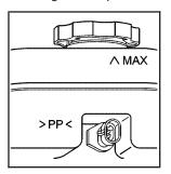
The fluid level should be above the PP mark. If it is not, have the brake hydraulic system checked to see if there is a leak.
